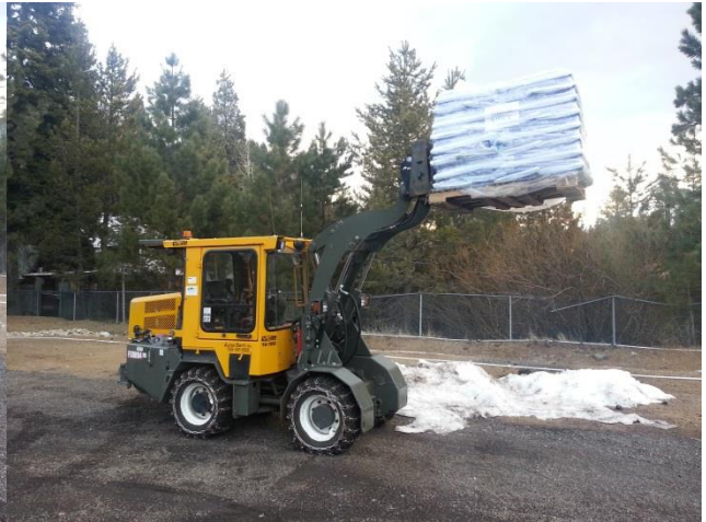
VTC TC-904 with Pallet forks with 2400lb pallet
