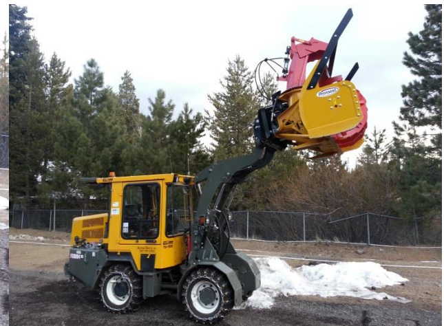
VTC TC-904 with Pallet forks with Pronovost PGS-800 snowblower
