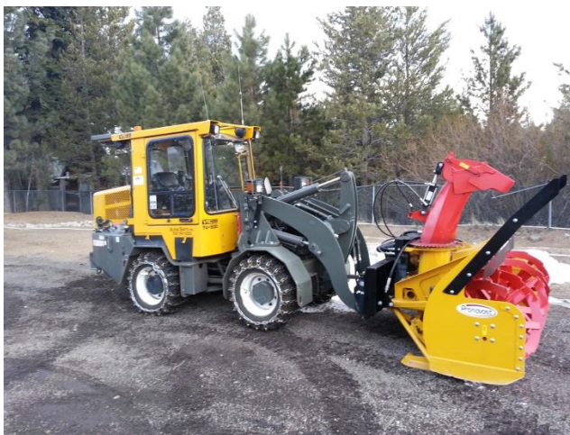
VTC TC-904 with Pallet forks with Pronovost PGS-800 snowblower
