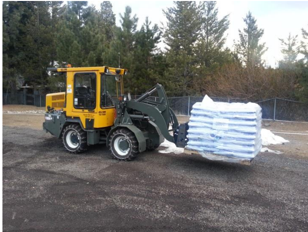
VTC TC-904 with Pallet forks with 2400lb pallet
