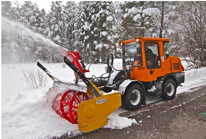
VTC 900-U with Pronovost PGS-800 Snow Blower
