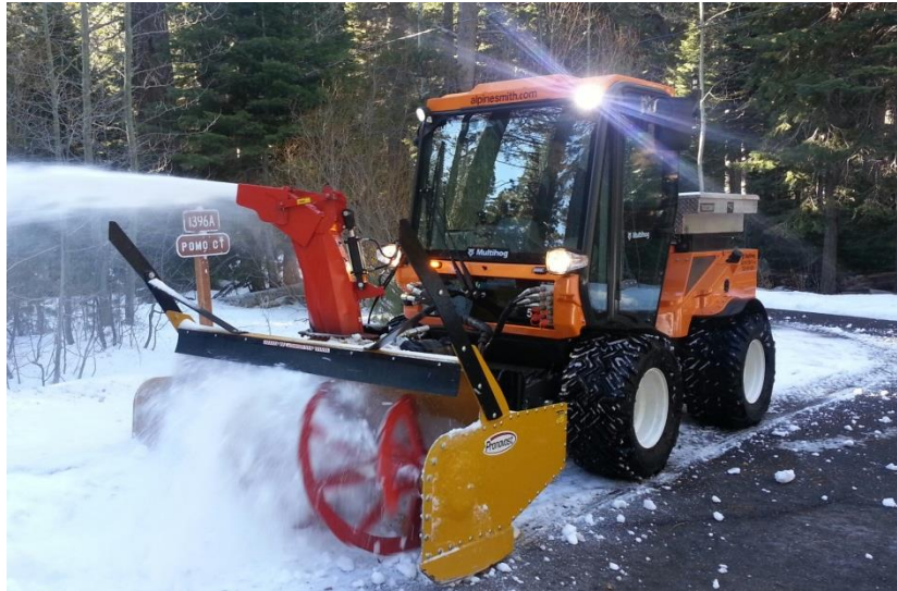
Multihog MH-90 with Pronovost PGS-800 Snow Blower
